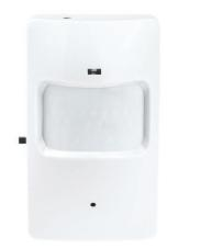
UltraLife series is designed for a long term surveillance usage. This module is equipped with low PIR sen-sor that allows you to monitor places with low activity movements for a long period of time. The module is placed manually to the covert PIR module, which makes it virtually unrecognizable from the real PIR module = sensor.
