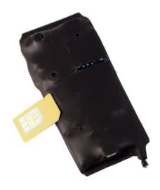
IMPORTANT: Stronic URP GSM K+ is a device which is a combination of 2 different modules, Listening module GSM based and then Voice Recording module with VOX activation only. To access the devices recordings, you have to connect it to a PC and physically get the data.
